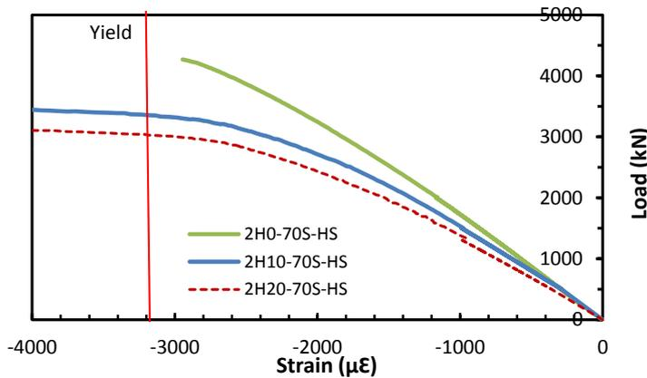
**Fig. 8** Load versus steel strain of 670 MPa longitudinal bar: (a) 200 × 200 and (b) 250 × 150 mm section.
