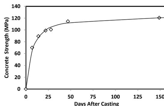
**Fig. 3** Concrete compressive strength versus days after casting.
