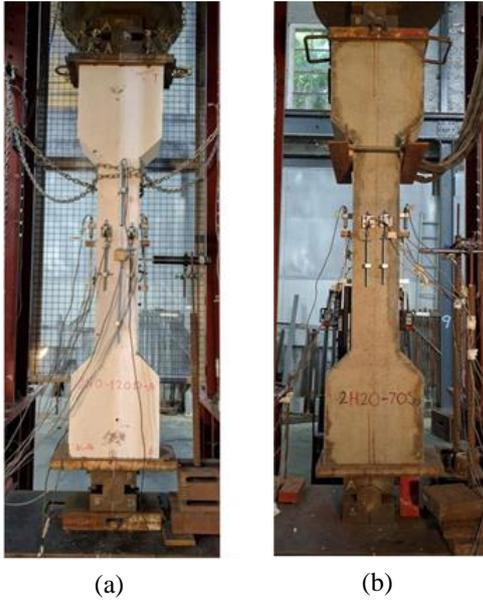
**Fig. 4** Testing arrangements: (a) concentric and (b) eccentric test set up.
