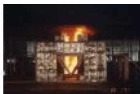
fire test on shoe storage area set-up
