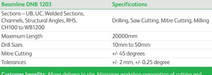
**Customer benefits:** Allows delivery to site. Minimises workshop preparation of cutting and drilling. Saves workshop time and space.
