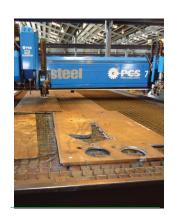
**Customer benefits:** High precision cutting and drilling including bevels with guaranteed accuracy (within tolerances) through CNC programmed parts. Etch and Pop marking to assist in bending and fabrication within the workshop.
