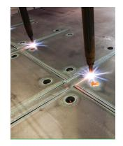
**Customer benefits:** Ideal for thicker plate material in larger sizes, multi-head cutting reduces time while CNC programing ensures accurate dimensions of all parts.
