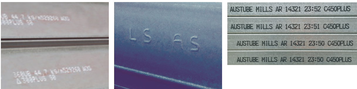
Pictured left to right, the unique identifiers for hot-rolled structural product and Austube Mills product.
