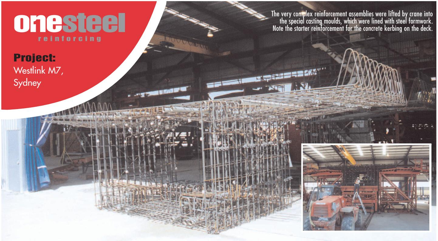
The very complex reinforcement assemblies were lifted by crane into the special casting moulds, which were lined with steel formwork. Note the starter reinforcement for the concrete kerbing on the deck.
