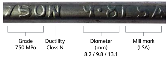
Figure 2. Typical rolled-in bar markings
