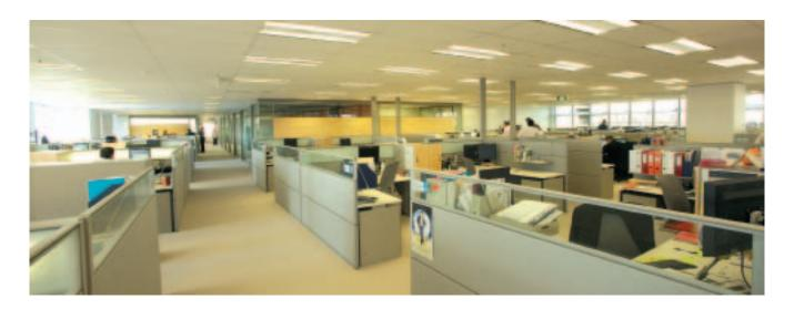
The column-free floor plate of the base building allowed the fit out design by Woods Bagot to incorporate a continuous subdivision module that allows all work point types to be interchangeable across the space and throughout the tenancy.
