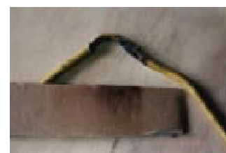
Conditions of PVC and cardboard after 12-13 minutes of exposure
