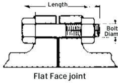
Steel hexagon Bolts and Nuts (XOX) are recommended for use within a temperature range of -50°C to +300°C. Outside of this temperature range, Stud Bolts should be used as recommended in AS.2528.
