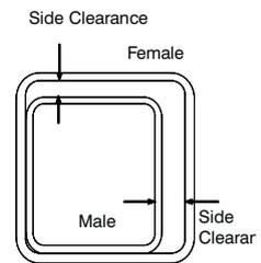
**Note:** SHS is not a precision tube and all dimensions shown in the chart, although in accordance with the specifications, may vary marginally within the tolerance bands permitted.
