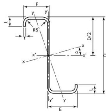
**Note:** Purlins are made from high tensile steel to be fastened rather than welded. Purlins can be ordered pre-cut to length and with pre-punched holes or slots.
