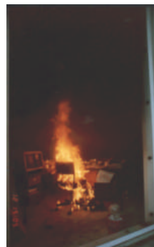
Fire just prior to the operation of the sprinkler
