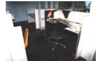
Extent of damage after Test 2
