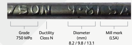
Figure 2. Typical rolled-in bar markings
