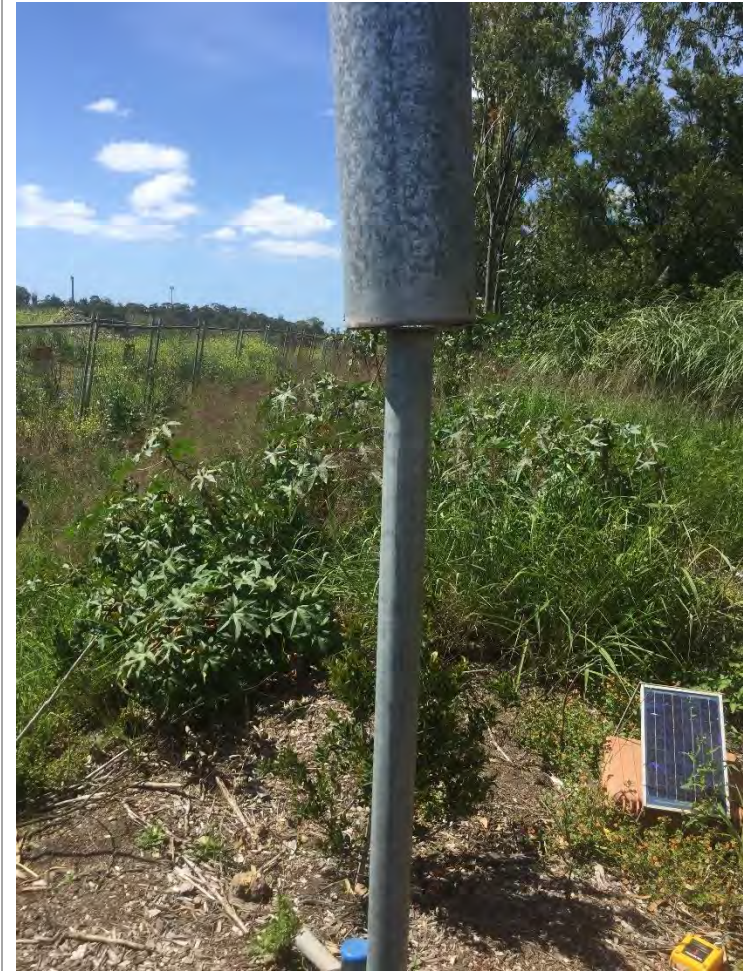
Photo 6 – Dust deposition gauge
