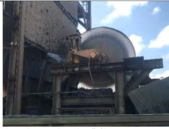
Figure 10 – Water Sprays installed in Drum Magnets
