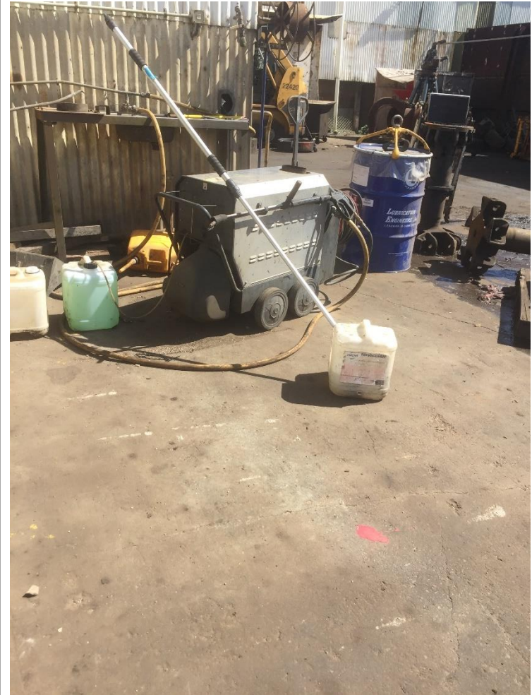
Photo 4 – Chemical containers not stored in a bunded area..
