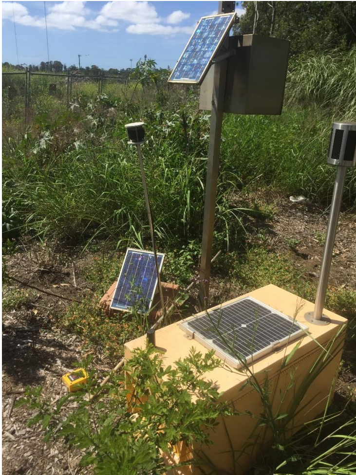
Photo 5 – Weather station and Blast and vibration monitor
