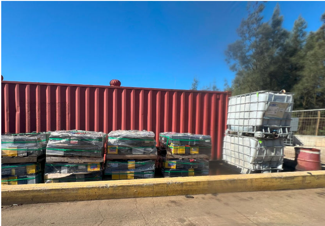
Plate P3. IBCs, drums and batteries stored in bunded area
