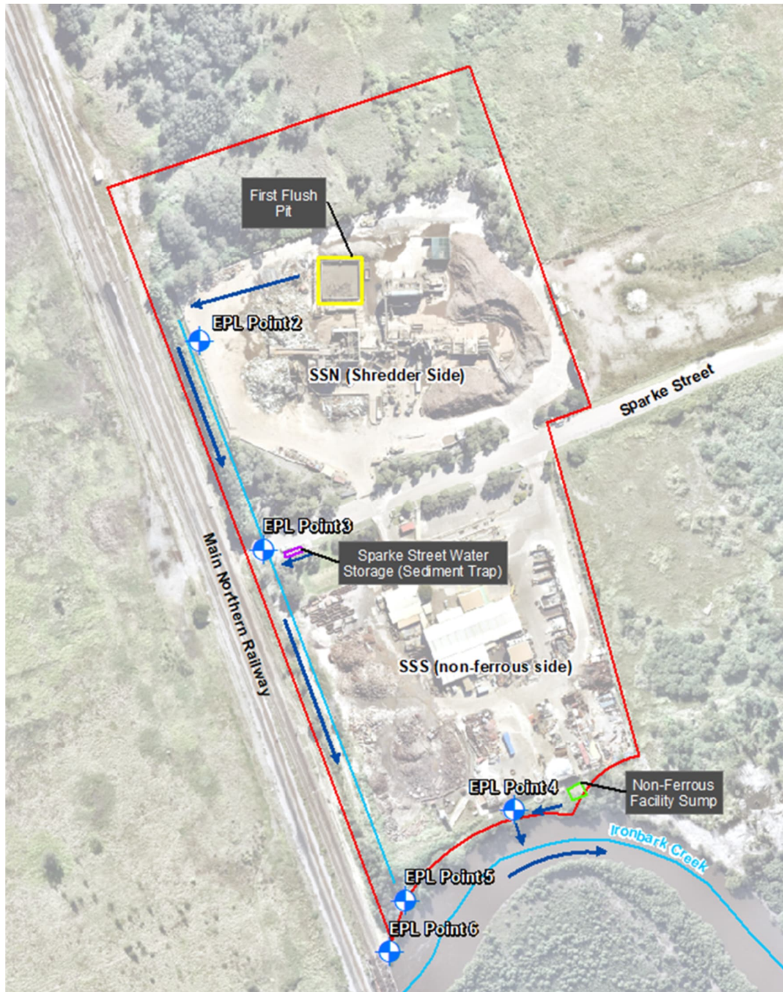
Figure 3 Surface Water Quality Monitoring Locations
